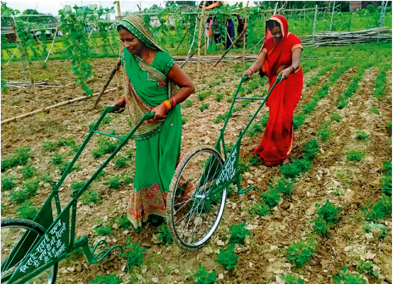
Women farmers using Cycle Weeder – a locally made innovative tool to reduce women’s drudgery in weeding crops. Photo: GEAG
