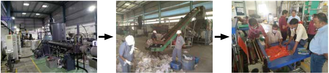
Figure 17: Washing plant (left), extrusion plant (center) and recycled plastic product manufacturing (right) at plastic recycling unit inside ISWM facility
