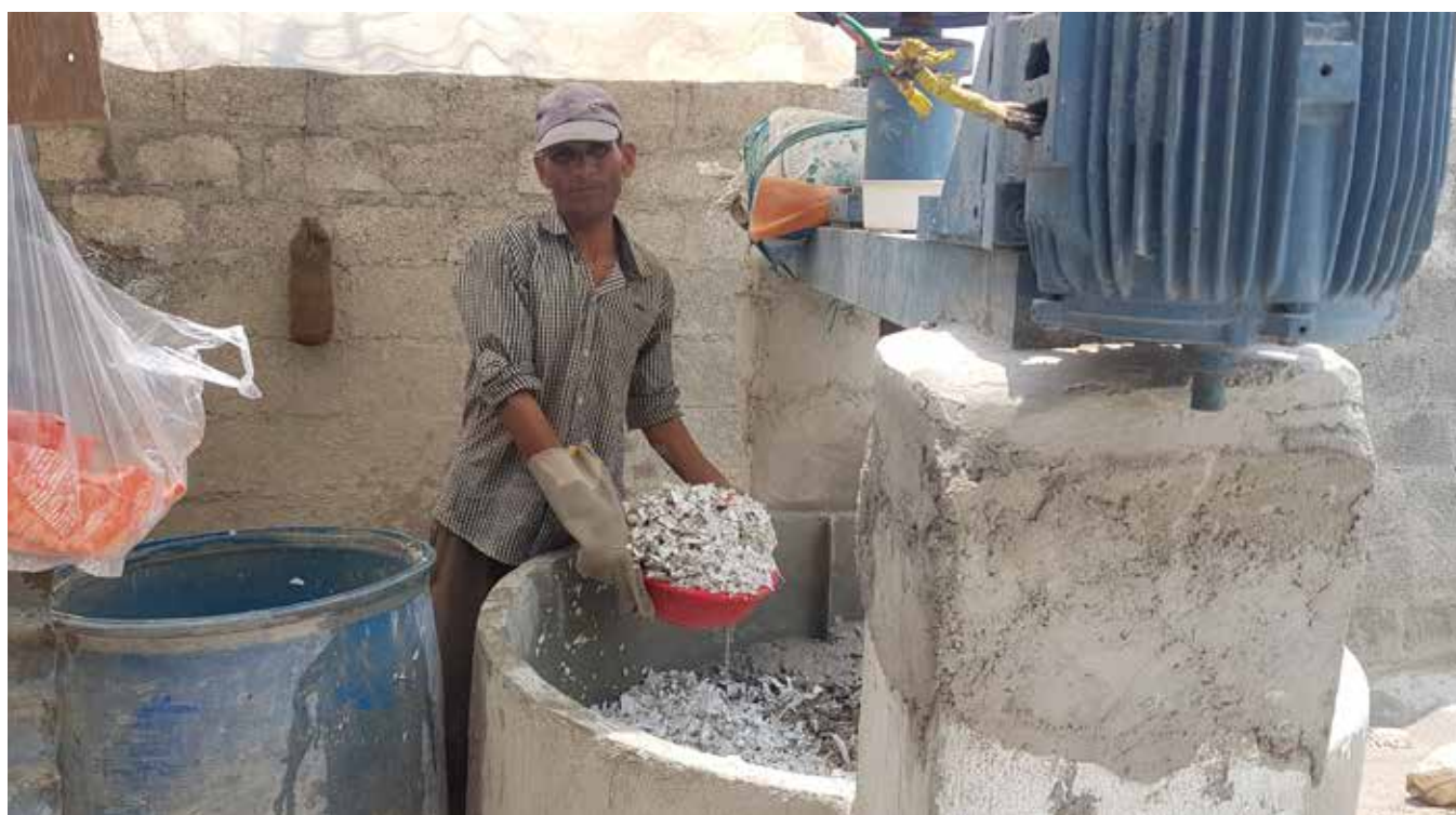
Figure 14: Semi-automated washing of shredded plastic
