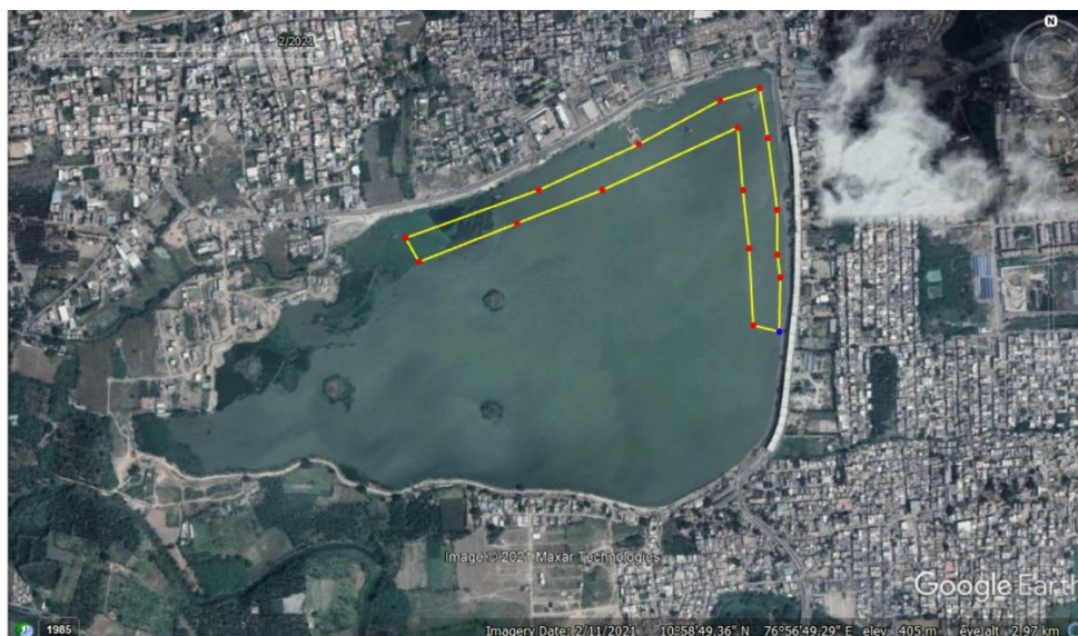
Figure 1 Area of Periyakulam Lake suggested by CCCMC for FSPV deployment
