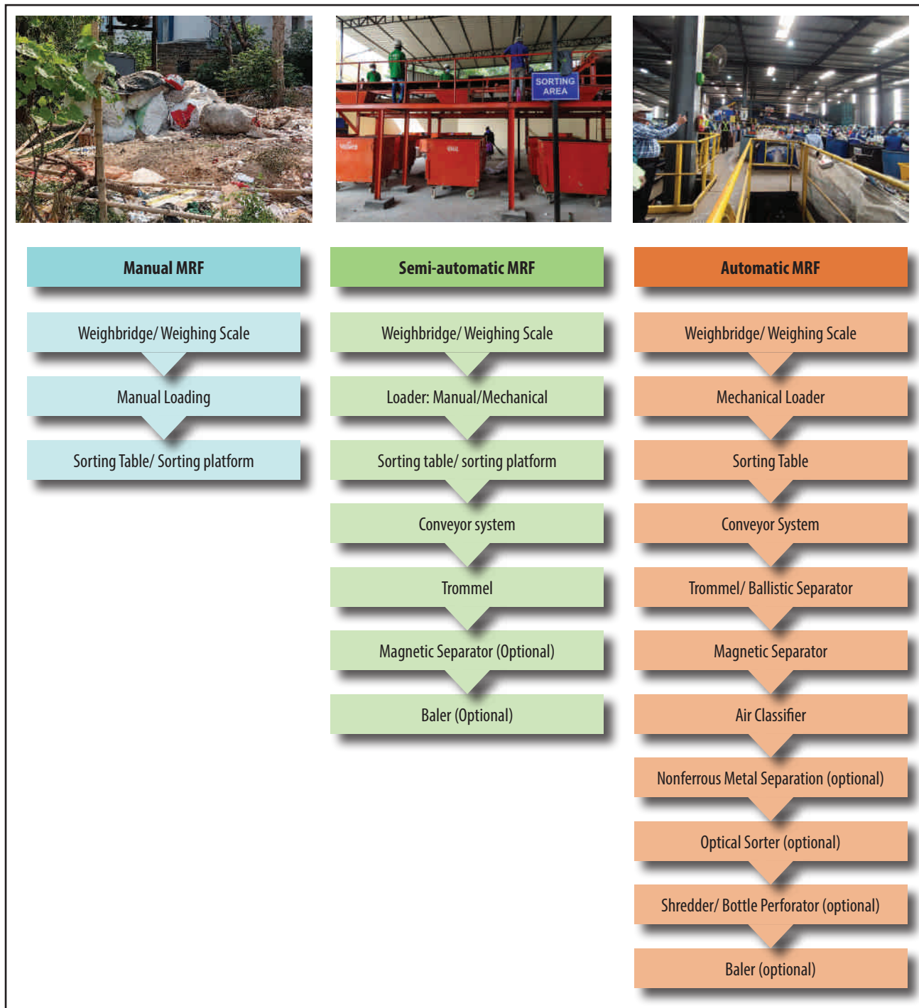
FIGURE 15: Comparison of Process Flow in Different Types of MRF (CPHEEO, 2020)
