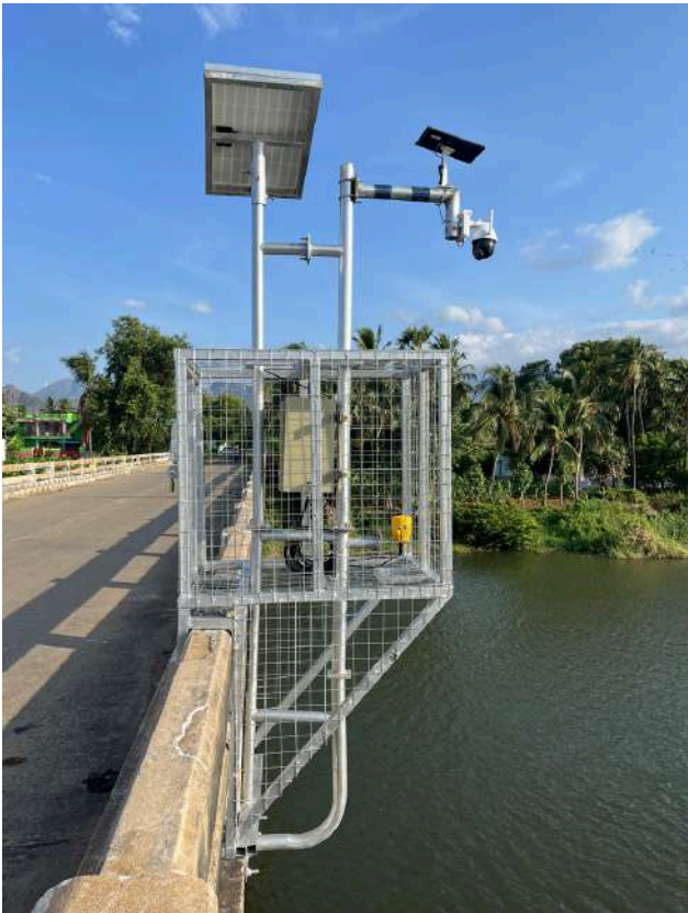
Installation of Bridge-Mounted Automatic Water Level Recorders as Flood Monitoring Sensors
