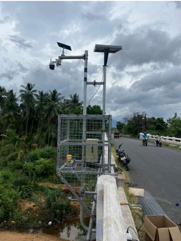
Installation of Bridge-Mounted Automatic Water Level Recorders as Flood Monitoring Sensors
