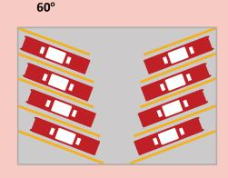
In this layout, buses are parked at an angle (typically 45 or 60 degrees) to the driving lane. It allows easier and quicker entry and exit for drivers compared to 90-degree parking. This setup strikes a good balance between efficient use of space and ease of maneuvering. (Wikipedia, 2025)
