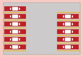
Buses are parked at a right angle to the driving lane. This layout maximizes the number of vehicles that can be accommodated in a given area. It is best suited for depots with ample space where bus movement is slower and more controlled.
