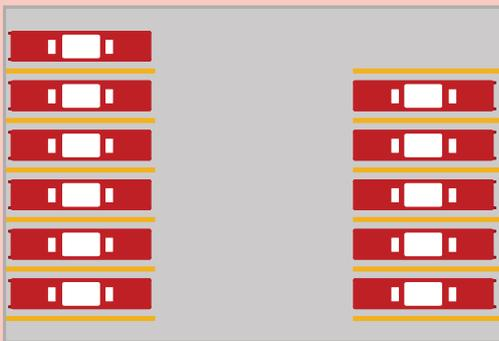
Buses are parked at a right angle to the driving lane. This layout maximizes the number of vehicles that can be accommodated in a given area. It is best suited for depots with ample space where bus movement is slower and more controlled.
