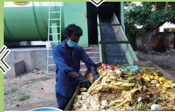
On-site processing of biodegradable (wet) waste in 1.5 TPD biomethanation plant
