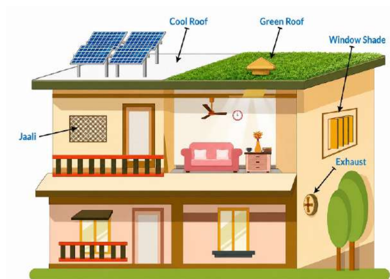
Figure 16: Illustration of Passive Cooling Strategies and Low-energy Comfort Systems
