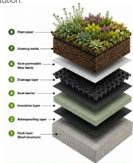
Figure 23: Green roof design
